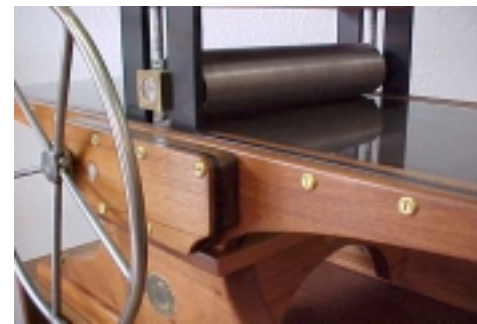
The Mariner has a gearbox that gives the user an 8:1 mechanical advantage so the wheel turns with ease.
